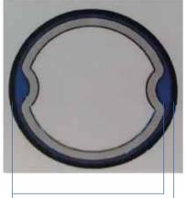
2 bigger air gaps makes airflow easier with result of low head los
